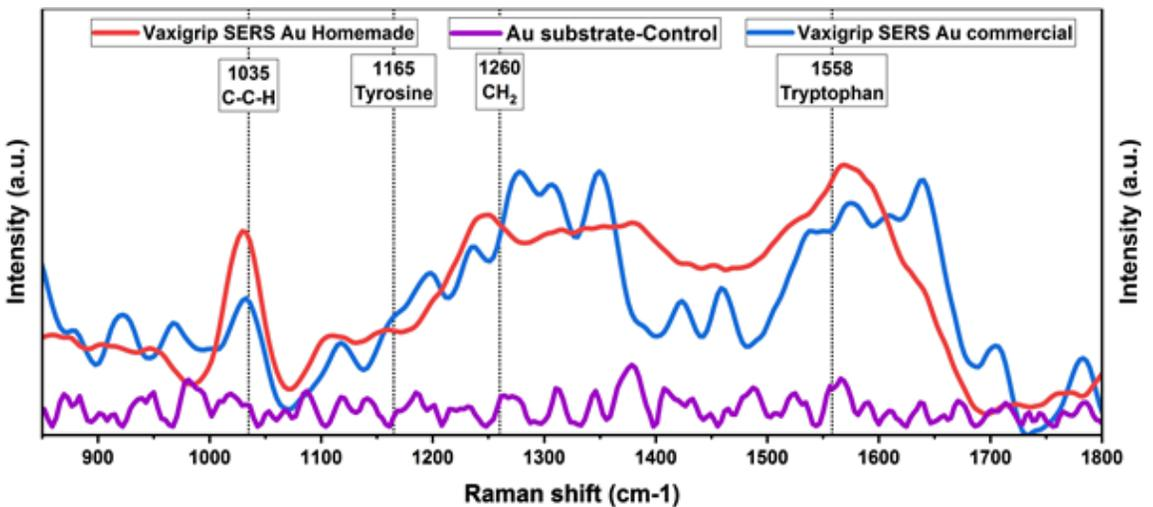
Figure 3: Raman spectra of a commercial influenza vaccine. These spectra were obtained using a commercial (blue line) and a homemade (red line) gold SERS substrates. The purple line shows the control spectrum for the measurement performed on the homemade SERS substrate.
