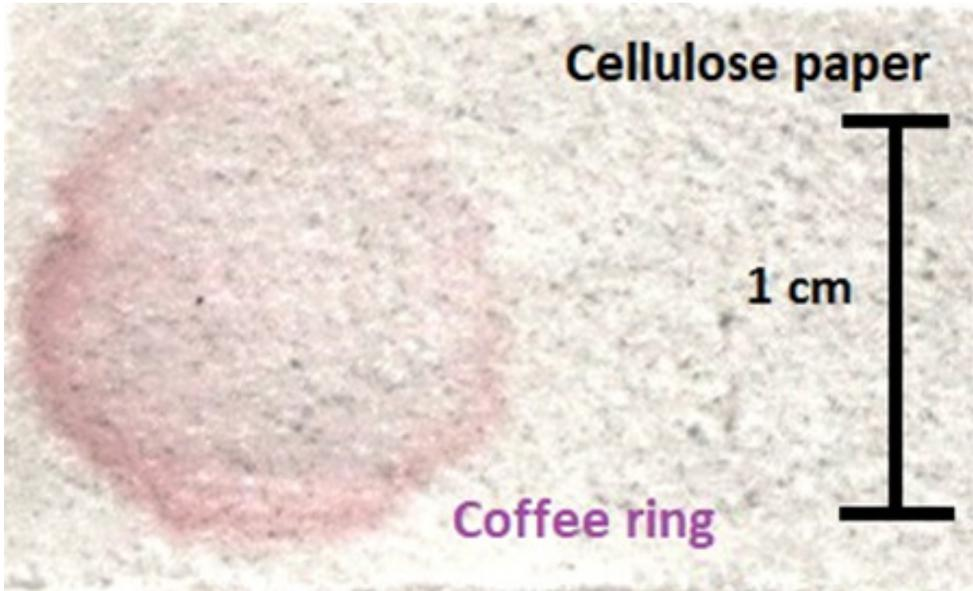
Figure 2: Photograph of an influenza vaccine sample on the homemade SERS substrate (gold nanoparticle+cellulosa paper). The coffee ring is clearly observed.
