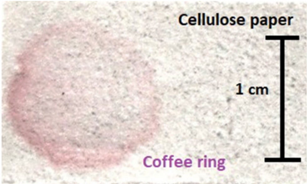
Figure 2: Photograph of an influenza vaccine sample on the homemade SERS substrate (gold nanoparticle+cellulose paper). The coffee ring is clearly observed.
